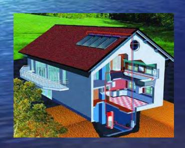
Example of small scale split solar water heater system.
