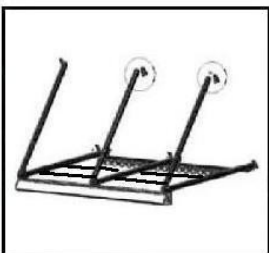
9. Install feet on the front legs and rear legs
