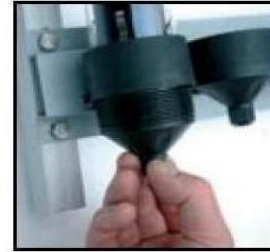
19. Circumgyrate and install the cap of tail stock tightly
