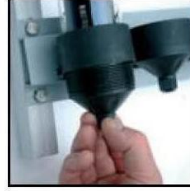
15. Circumgyrate and install the cap of tail stock tightly
