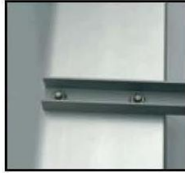
2. Tighten nuts between the front legs and manifold
