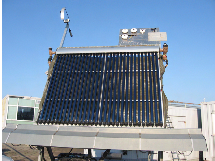
Figure 1: Picture of the collector TZ58-1800-30R mounted on the test facility of Fraunhofer ISE
